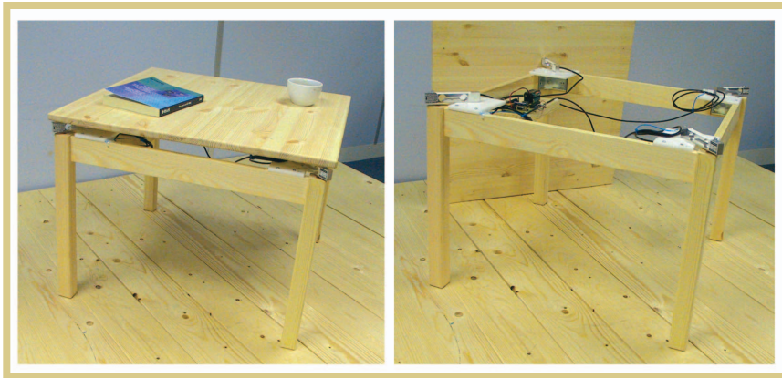
Figure 8. We can (a) transform a regular coffee table into an interactive and context-sensitive device by (b) unobtrusively embedding Smart-Its and load sensors.
