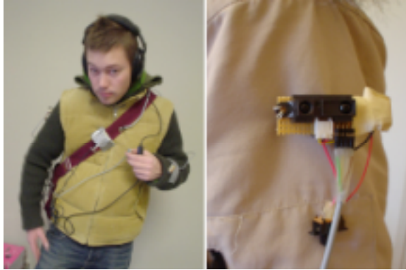
Figure 2: a) User wearing the Sonic City prototype; b) proximity IR-sensor on another user's arm
