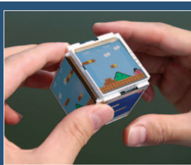
Figure 1. The Z-Agon concept is an innovative display device in the form of a cube.
