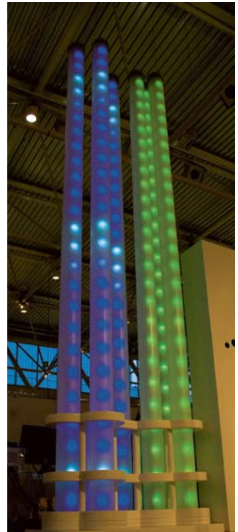
Six frosted Plexiglas tubes, four meters tall, suspended from the ceiling in an arrangement borrowed from the Lyra star constellation. There are 50 led-based RGB lights in each tube. The construction can be seen as a 300 pixel display with 900 control channels conducted by our own software. As Lyra floats in the Electrum space in May 2008, its behaviour will reflect activities in the building. We will also produce an interface giving visiting artists the possibility to design their own graphics and animations.
