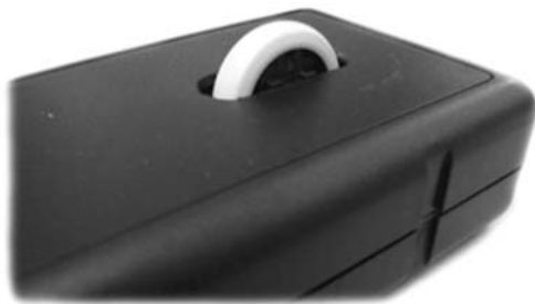
Fig. 4. The small wheel built on parts from a mouse.
