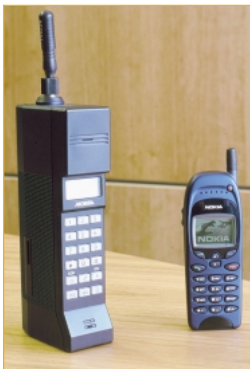
Figure 1: The Mobira Cityman, a Nokia Mobile Telephone from the 1980s (left) and the Nokia 6110, a cellular phone from the late 1990s (right)
