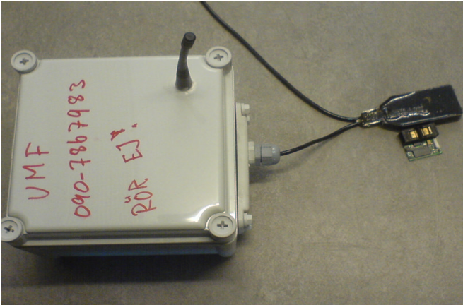
Fig. 6. Encapsulated node and simple buoy
