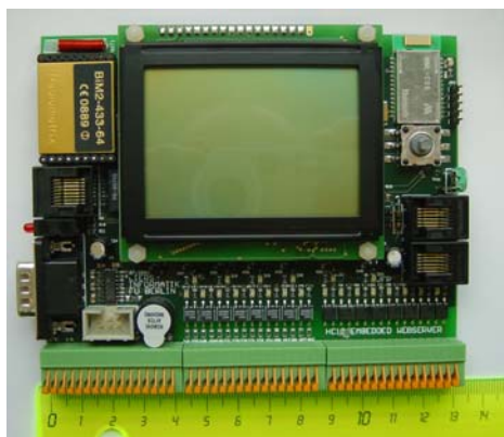
Figure 1. Embedded Wireless Module
