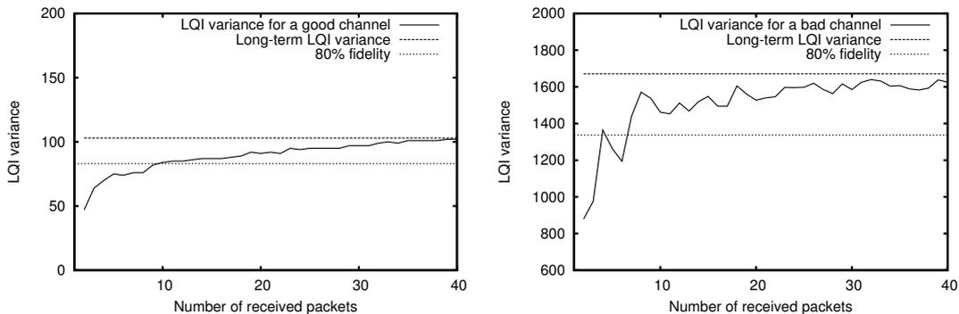
**Figure 1: LQI variance for a channel with high PRR (good) and a channel with a lower PRR (bad). The left figure shows the good channel (PRR of 99.9%) with LQI variance of about 100, while the LQI variance of the bad channel (PRR of 87%) in the right figure is around 16 times higher.**
